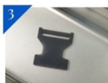
3 Final rinse for 3 minutes in ultrasonic cleaner.
